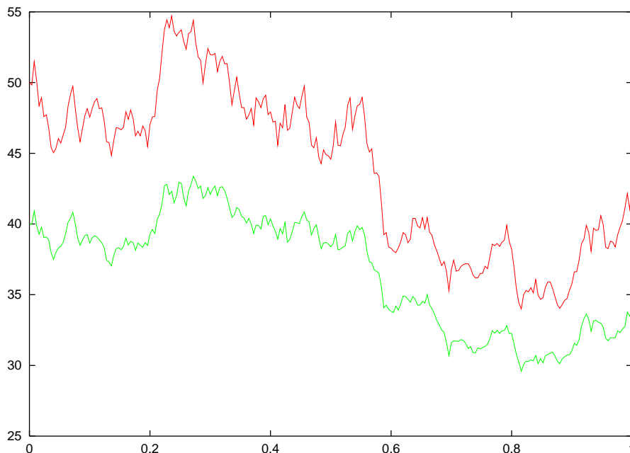
Fig. 2.7. Simulation of a correlated vector process with two components, and \mu = 0.05 , \sigma_1 = 0.3 , \sigma_2 = 0.2 , \rho = 0.85 , \Delta t = 1/250
